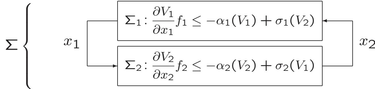
iISS-ISS interconnection:  $\alpha_1(s) = \frac{s}{s+1}$ ,  $\sigma_1(s) = \frac{5s}{4s+6}$ ,  $\alpha_2(s) = s$ ,  $\sigma_2(s) = \frac{5s}{7s+6}$
